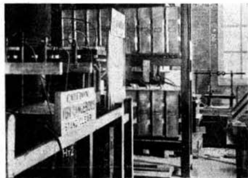
Some of the early apparatus at the Poldhu wireless station, used in sending the first transatlantic wireless signals. On the left are the transformers; banks of condensers are carried in metal containers on the wooden rack (centre); and on the extreme right is the spark-gap, consisting of two steel spheres mounted on insulating rods.
